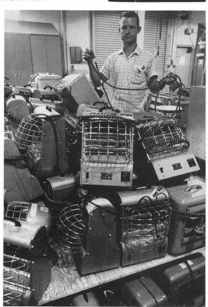
ELECTRIC HEATERS, called in last week by Plant Engineering Department 4540, are piled high awaiting complete checking and overhaul by electricians in 4511-2. Frayed cords, such as the one held by Billy D. Thompson above, will be replaced along with other defective parts. All heaters should be turned in to Division 4542, Bldg. 887, ext. 21158.
